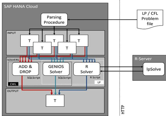
Figure 1. Solution architecture
