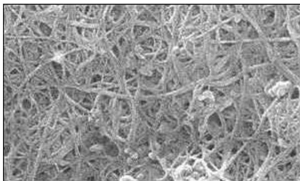
This "paper" is made of nanotubes and contracts when charged. It has been shown that the tiny nanotubes expand and contract their length by about 1% when an electric charge is applied and then removed (3).
