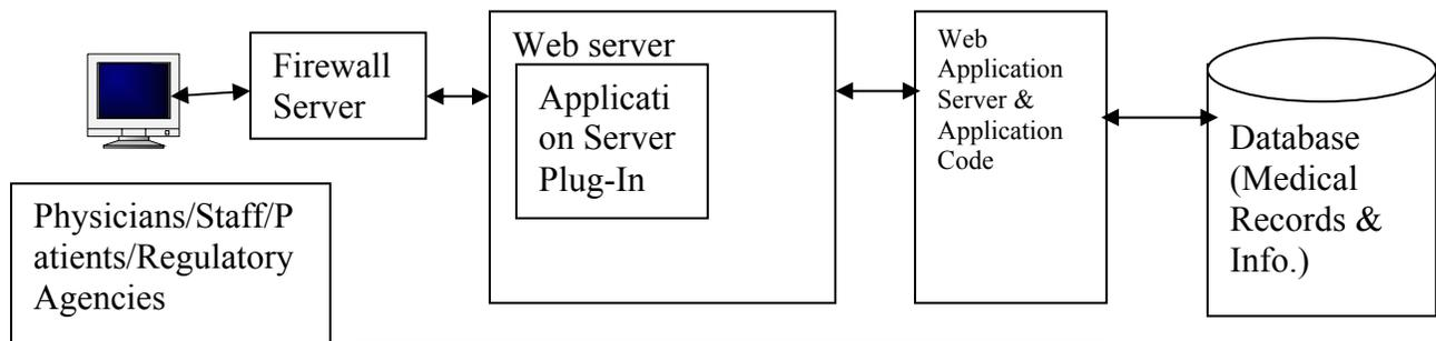
Figure 1: General thin-client architecture.
