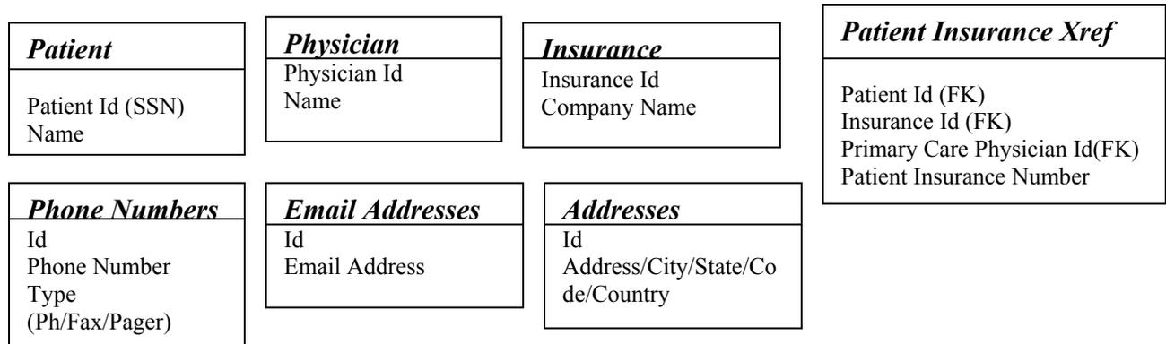
Figure 2: Basic database tables for the Medical Information System.
