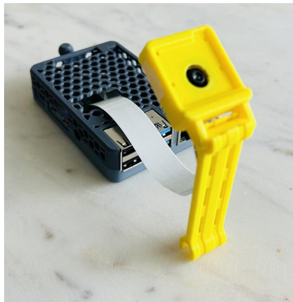
Fig. 9. Shows Raspberry Pi 4 and Pi camera module used to run the real-time traffic sign detection system.
