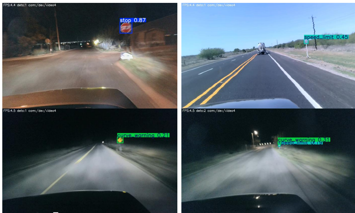
Fig. 11. Additional real-world detection outputs. Top Left: Stop Sign at night (conf: 0.87). Top Right: Speed limit 60, highway daytime (conf: 0.45). Bottom Left: curve warning, nighttime (conf: 0.21, due to foggy weather and motion blur). Bottom Right: curve warning and speed limit 15 (conf: 0.31 and 0.19, due to sign distance, motion blur, and foggy weather).
