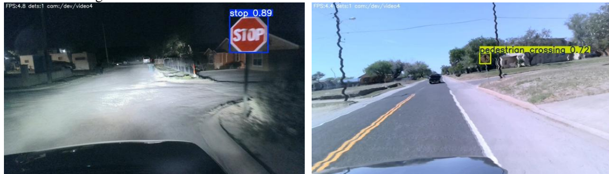
Fig. 10. Real-world detection outputs. Top: nighttime stop sign (conf: 0.89). Bottom: daytime pedestrian crossing (conf: 0.72). System running at ~4.8 FPS on Raspberry Pi 4.
